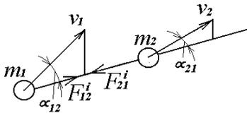
$$\begin{aligned} \sum dA^i &= F_{12}^i v_1 dt \cos \alpha_{12} - F_{21}^i v_2 dt \cos \alpha_{21} = \\ &= F_{12} (v_1 \cos \alpha_{12} - v_2 \cos \alpha_{21}) dt = 0 \end{aligned}$$
