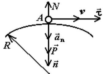
$$ma_n = \sum F_{kn}, \quad a_n = \frac{v^2}{R}; \quad \sum F_{kn} = P - N = mg - N; \quad m \frac{v^2}{R} = mg - N;$$
