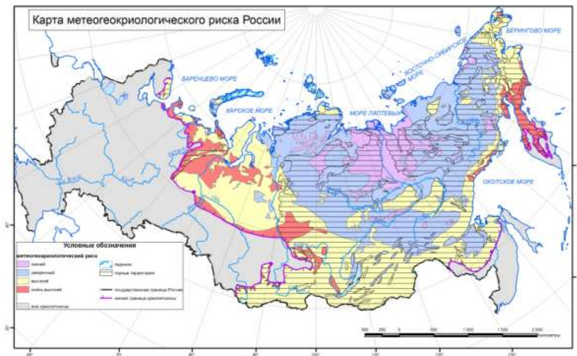
Map of zoning of the Russian territory according to the meteorological hazard for permafrost (red colour – maximal risk, violet colour – minimal risk)
